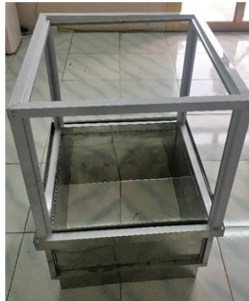
*Proposed GHG Measurement Chamber Design*
