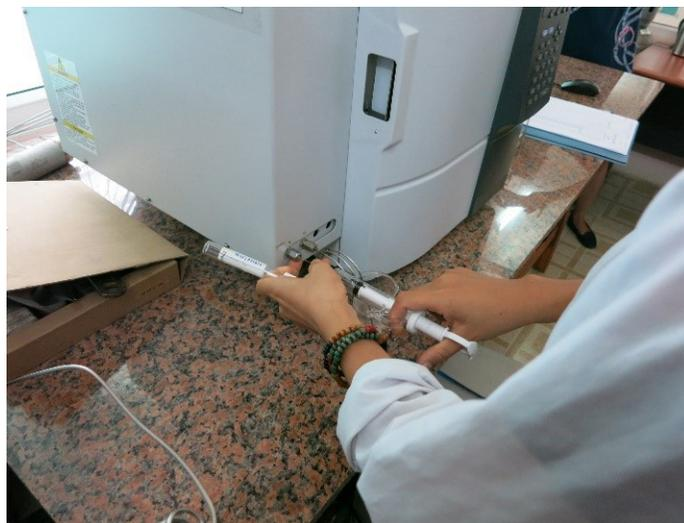
Figure 3: Preparing a Gas Sample for GHG Analysis
