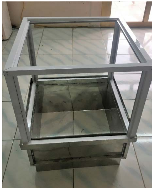
Model for a static GHG measurement chamber
